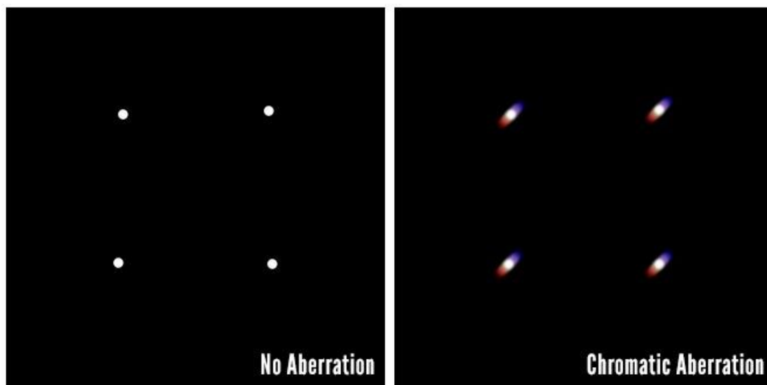
Diagram 4: Illustrating chromatic aberration
