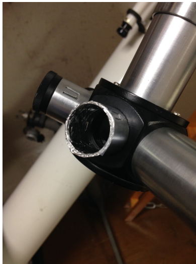
Diagram 5: Aluminium foil around unitron lens to eyepiece adapter
