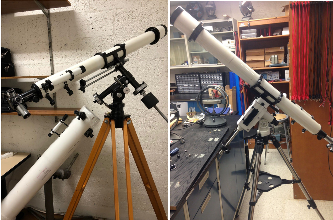
Diagram 9: Before-with wooden tripod mount After-with iOptron SmartEQ Pro+ mount
