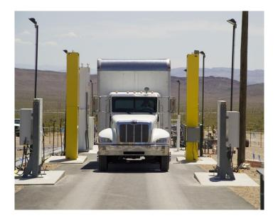
Figure 1.15: A truck going through a portal monitor [31].
