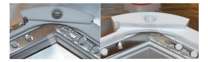
Figure 2.16: Close-up view of the recess created where the anode voltage connects to the frame. The connector is threaded Teflon with a brass "bullet" that connects to the anode wire. Some of the connector components are visible in the left picture. In the left and the right the threaded posts that attach the anode to the spacer are shown. These were held in place by delicate Teflon nuts, all of which were very susceptible to stripping.
