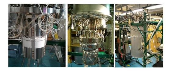
Figure 2.5: "Russian doll" images of PIXeY. Left image: inner detector showing to PMT block, bottom PMT block, and field region. Middle: Stainless steel outer can which form fits around the inner region, in order to keep the amount of liquid xenon used to a minimum. Right: Outermost can which insulates the inner can. The operational temperature of the detector is 175K, which liquefies the xenon.
