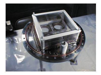
Figure 1.13: View of the inner region of LXeGRIT. The device was built to survive balloon flights.
